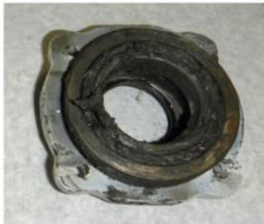
Figure 15 – Gearbox Upper Thrust Bearing with Grease, but Dry and Stiff
