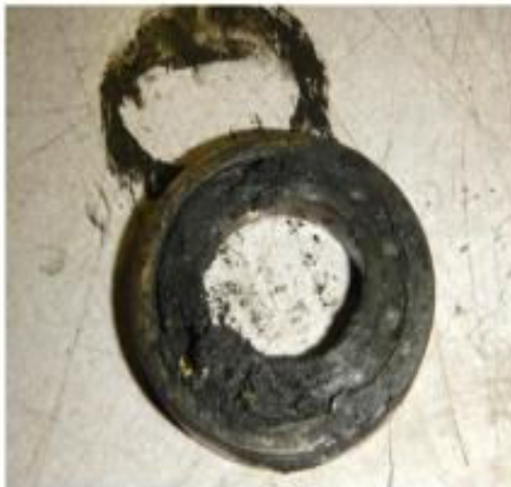
Figure 13 – Gearbox Lower Bearing with Grease, but Dry and Stiff
