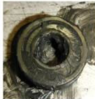
Figure 20 – Outer Pinion Bearing with Grease, but Thick and Gummy
