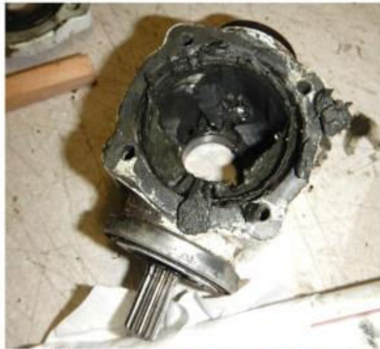
Figure 11 – Actuator Housing with Grease but Dry and Stiff
