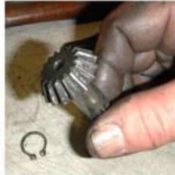
Figure 18 – Pinion Gear with Grease, but Dry and Stiff
