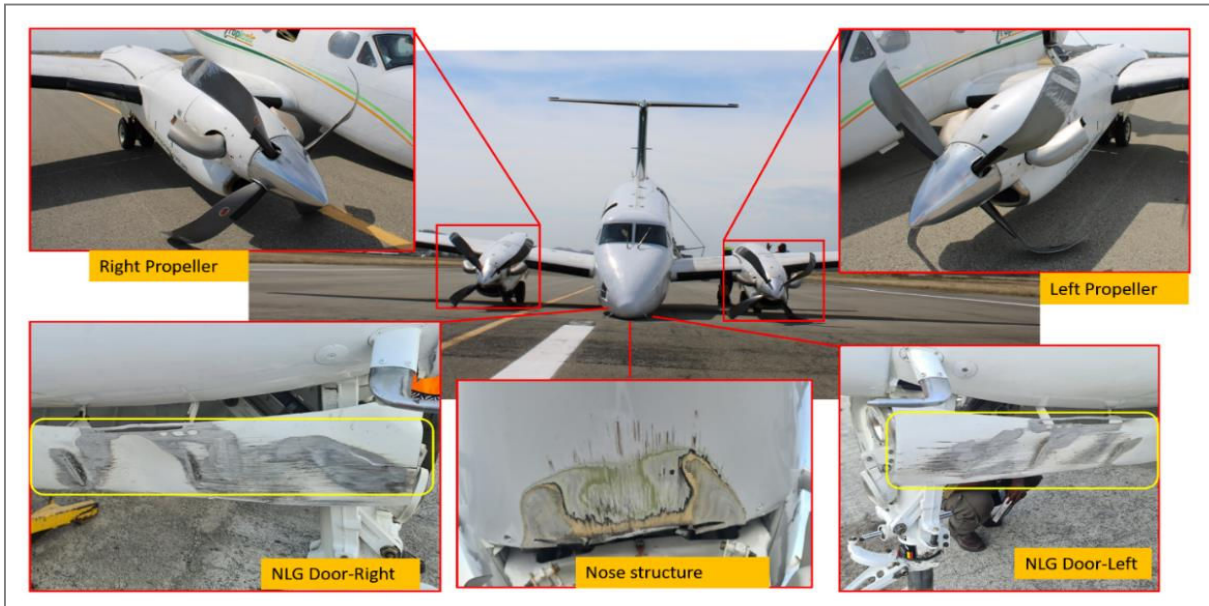
Figure 15:P2-JAU Overview of Damage Sustained.
