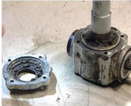
Figure 10 – Top Cover and Gearbox Upper Thrust Bearing with Grease
