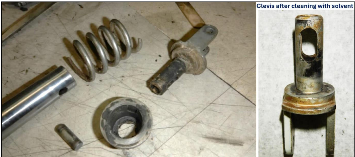
Figure 23: Clevis Pin, Clevis Spring and Retainer.
