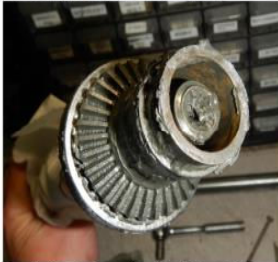
Figure 12 – Actuator Screw Assembly with Grease but Dry and Stiff
