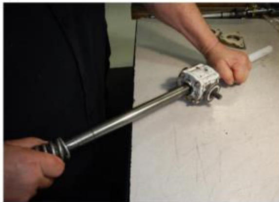
Figure 6 – Nut Assembly Removal Without Rotation
