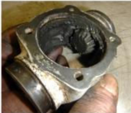
Figure 17 – Pinion Gear with Grease, but Dry and Stiff
