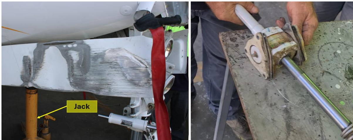
Figure 16:Retraction Test of the NLG and Inspection of the Faulty Actuator at Tropicair Hangar.
