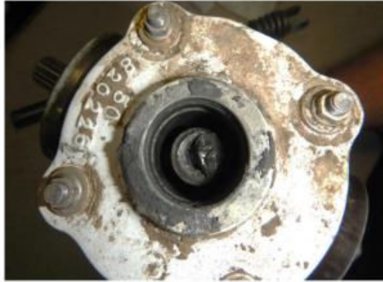
Figure 8 – Screw with Grease
