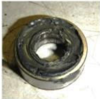
Figure 19 – Inner Pinion Thrust Bearing with Grease, but Thick and Gummy
