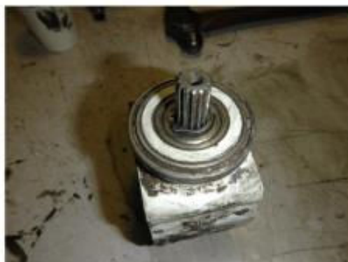
Figure 16 –The External Spline Gear Portion of the Pinion Gear Prior to Removal
