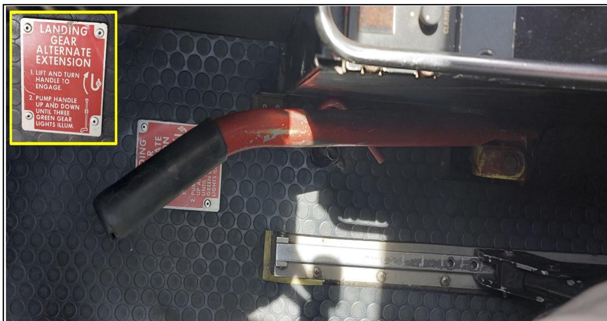
Figure 9:P2-JAU Mechanical Landing Gear Alternate Extension-Manual Control.
