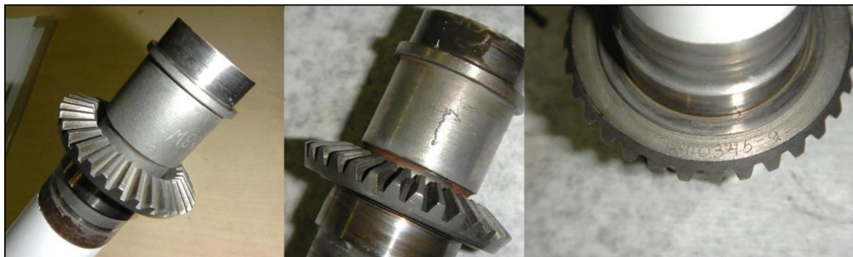
Figure 21: Bevel Gear Teeth.
