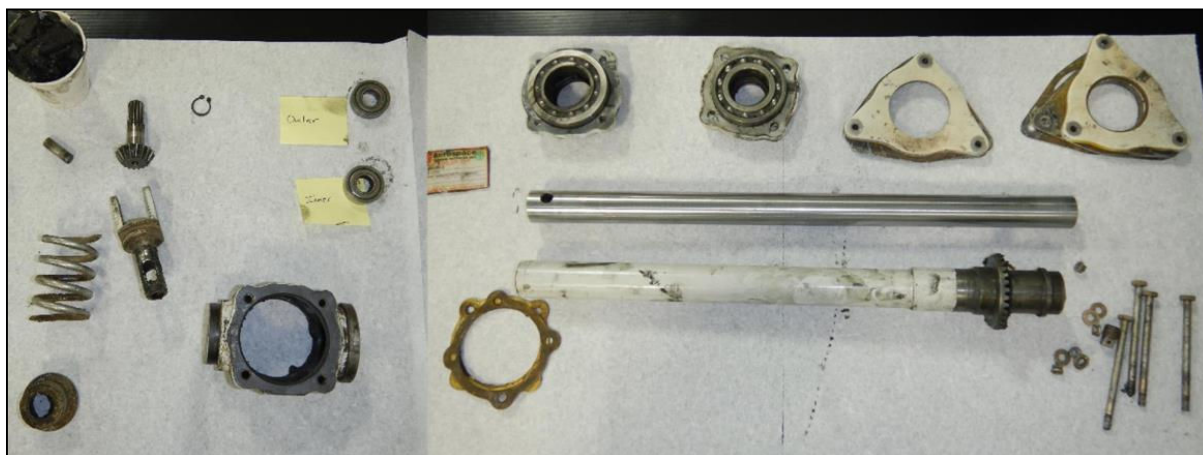
Figure 20: Components cleaned with solvent for further examination.
