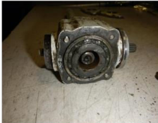
Figure 9 – Gearbox Lower Bearing with Grease
