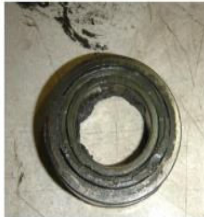
Figure 14 – Gearbox Lower Bearing with Grease, but Dry and Stiff, Other Side
