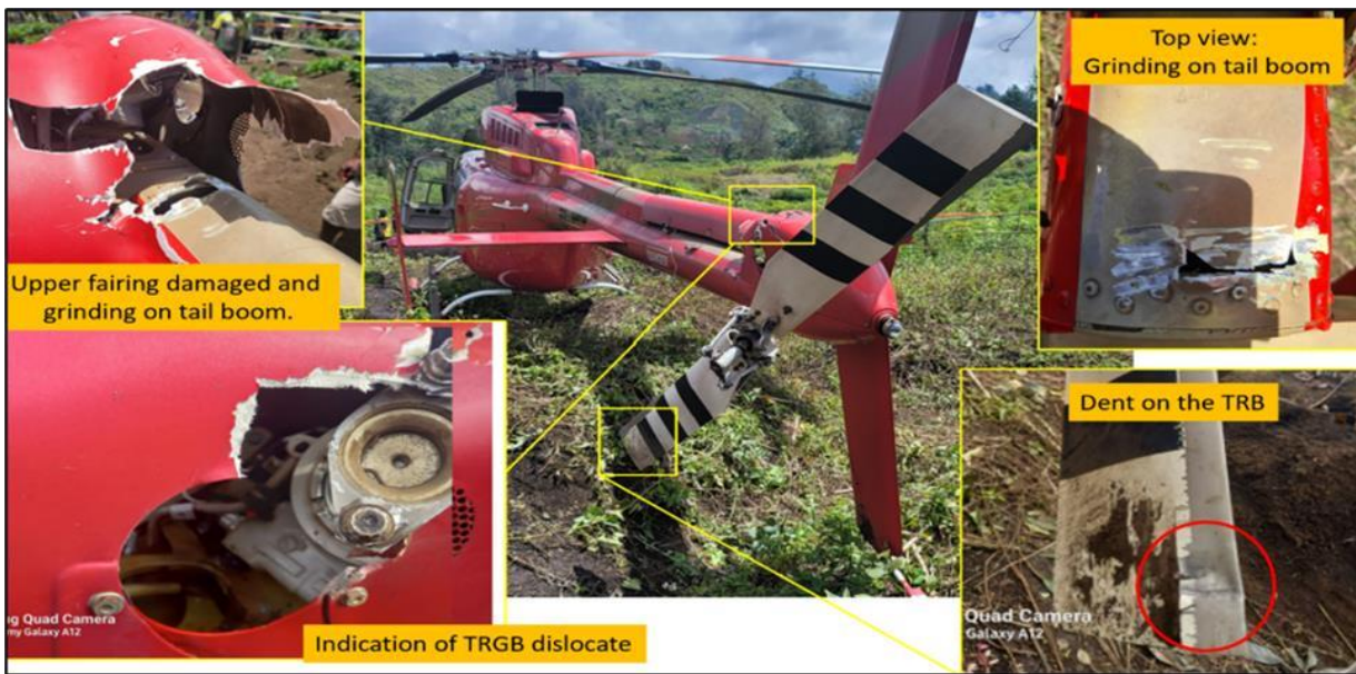
Figure 11: Damage sustained to the TRGB and Tail Boom
