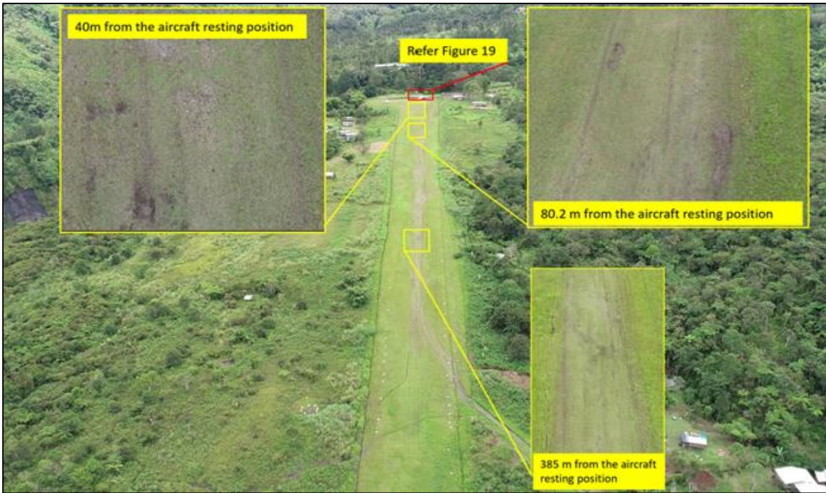
Figure 16:P2-HFA tyre marks along runway 14.
