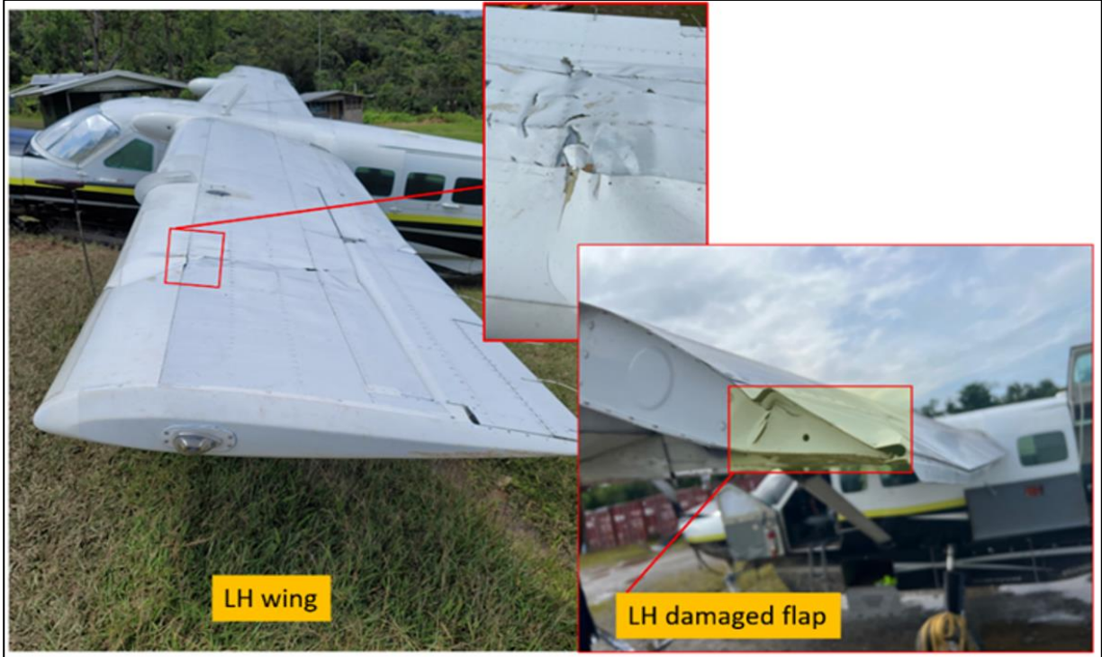
Figure 21:Damage to the LH wing and the LH wing flap.
