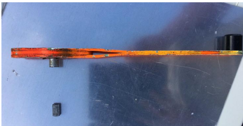
Figure 2: Broken landing gear manual extension pump handle
