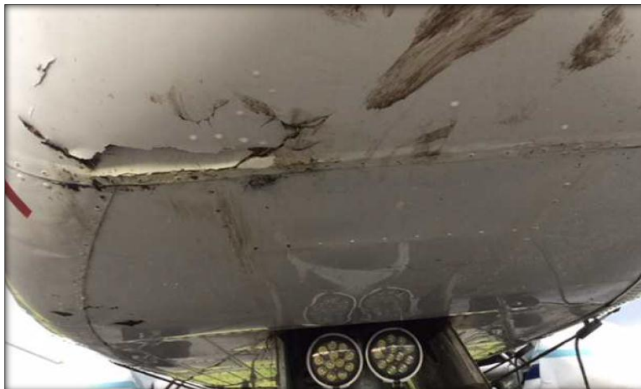
Figure 4: Puncture hole on the underside of the Nose Cone
