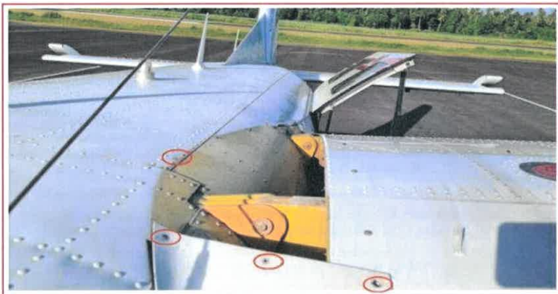
Figure 6: Screws missing from locations circled in red.
