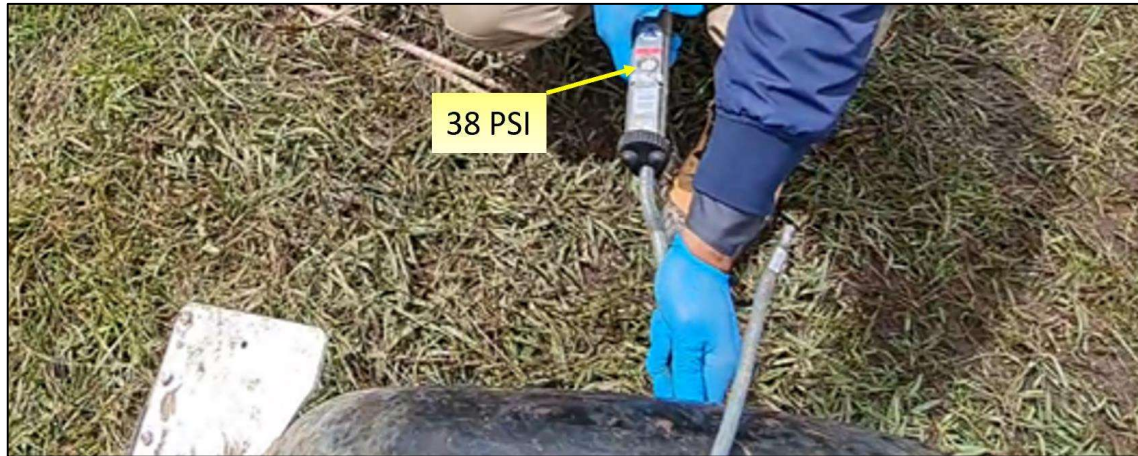
Figure 13: Evidence of sufficient pressure in the left main landing tire
