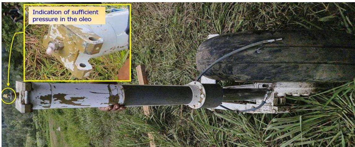
Figure 12: Evidence of sufficient pressure in the oleo strut
