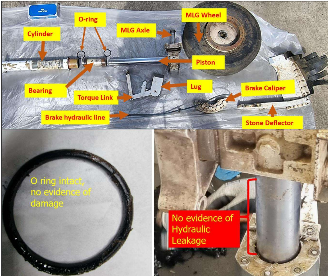
Figure 15: Left MLG Disassembly
