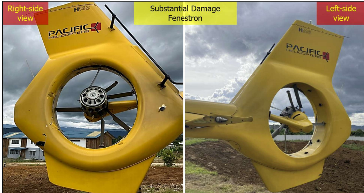
Figure 4: Fenestron substantially damage
