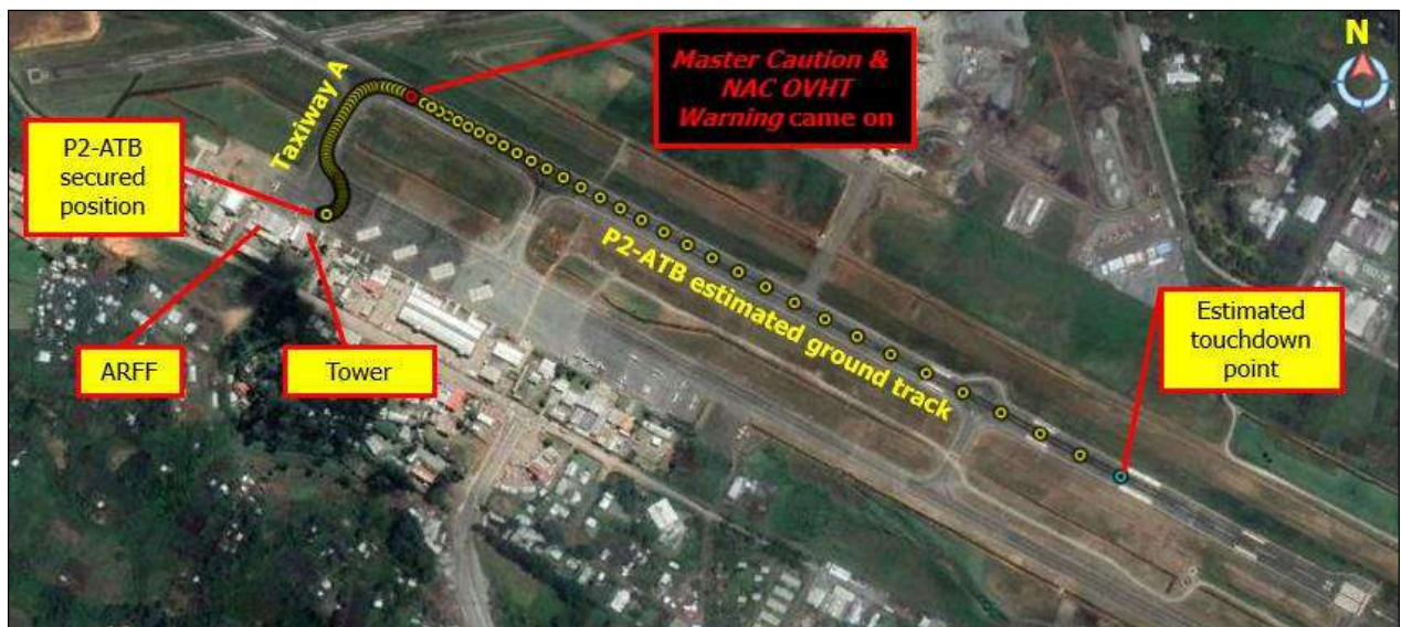
Figure 3: Derived ground track of P2-ATB after touchdown with significant events.
