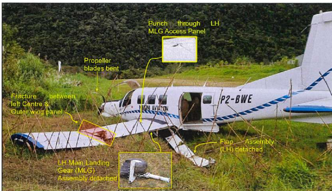
Figure 3: Overview of the damage sustained during impact
