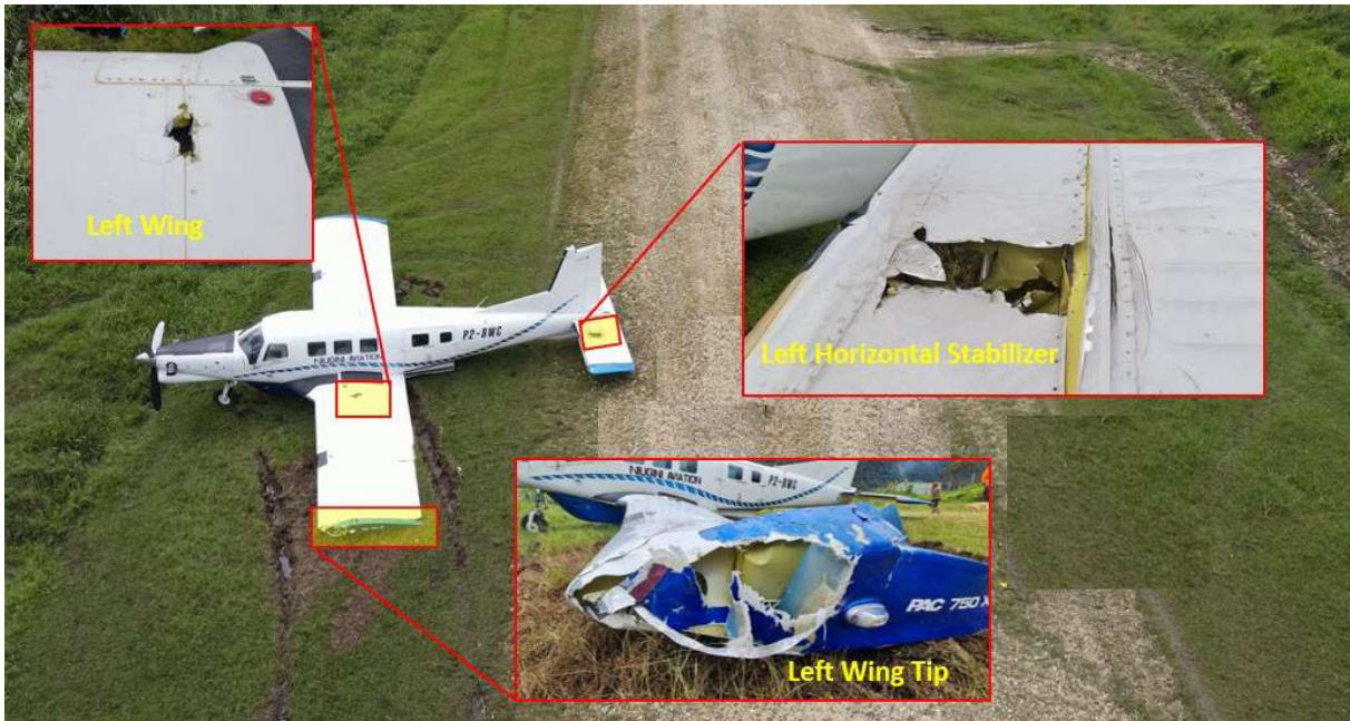
Figure 4: Overview of the damage sustained on P2-BWC
