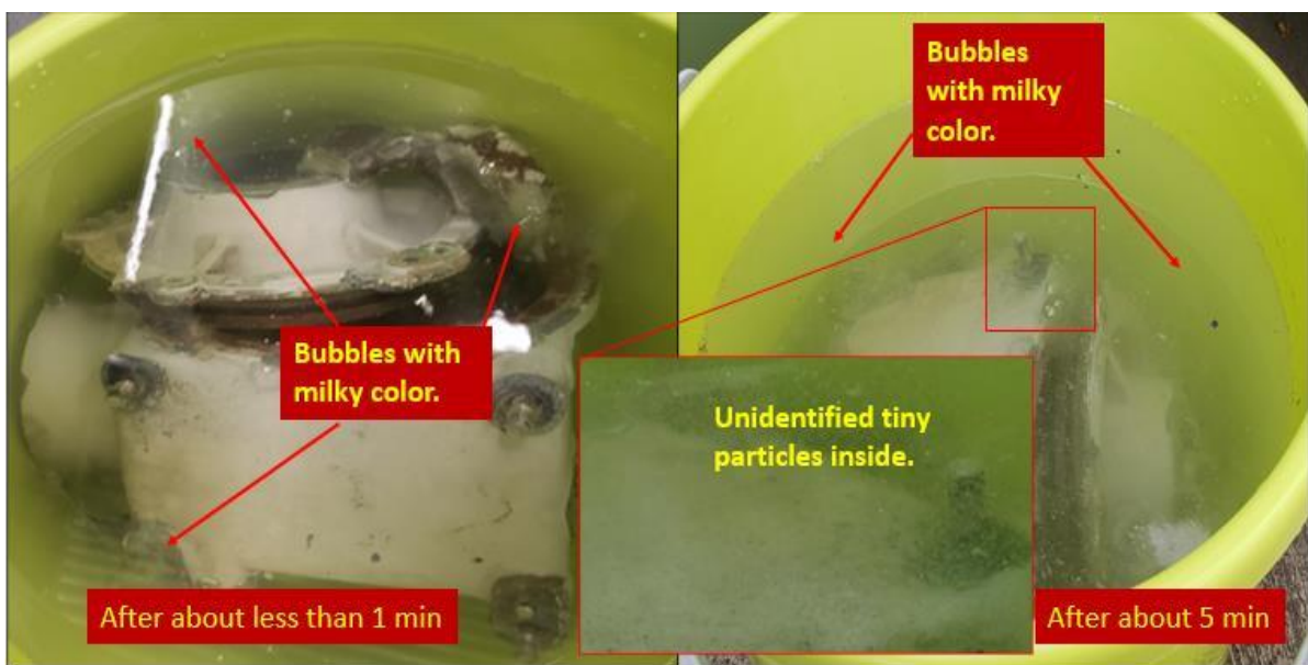
Figure: 13. Reaction of tail rotor gearbox housing with salt water at different times
