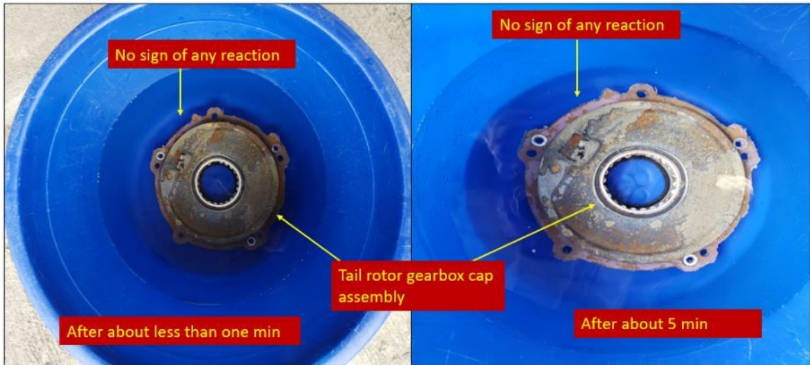
Figure: 15 Reaction of tail rotor gearbox cap assembly with fresh water at different times
