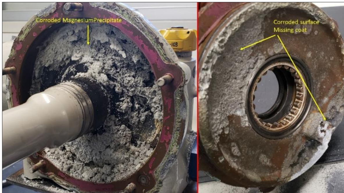
Figure 11: Corroded inner tail rotor gearbox housing
