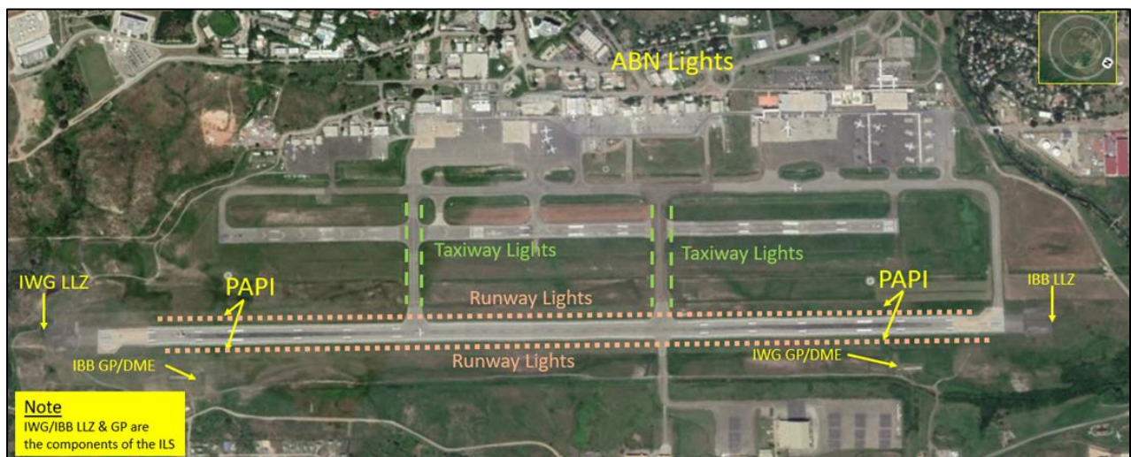
Figure 1: Some of the services were affected during the power outage
