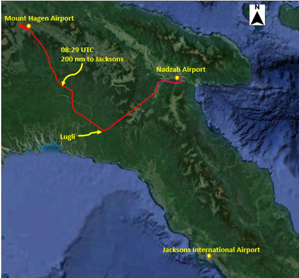
Figure 4: P2-ATC Flight Track highlighting the position where the aircraft was notified about the power outage
