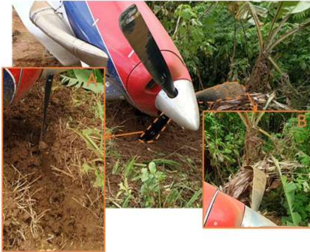
Figure 9: All propeller blades showing evidence of contact with ground. A – propeller dug into the ground, B – propeller significantly bent due post impact with ground.
