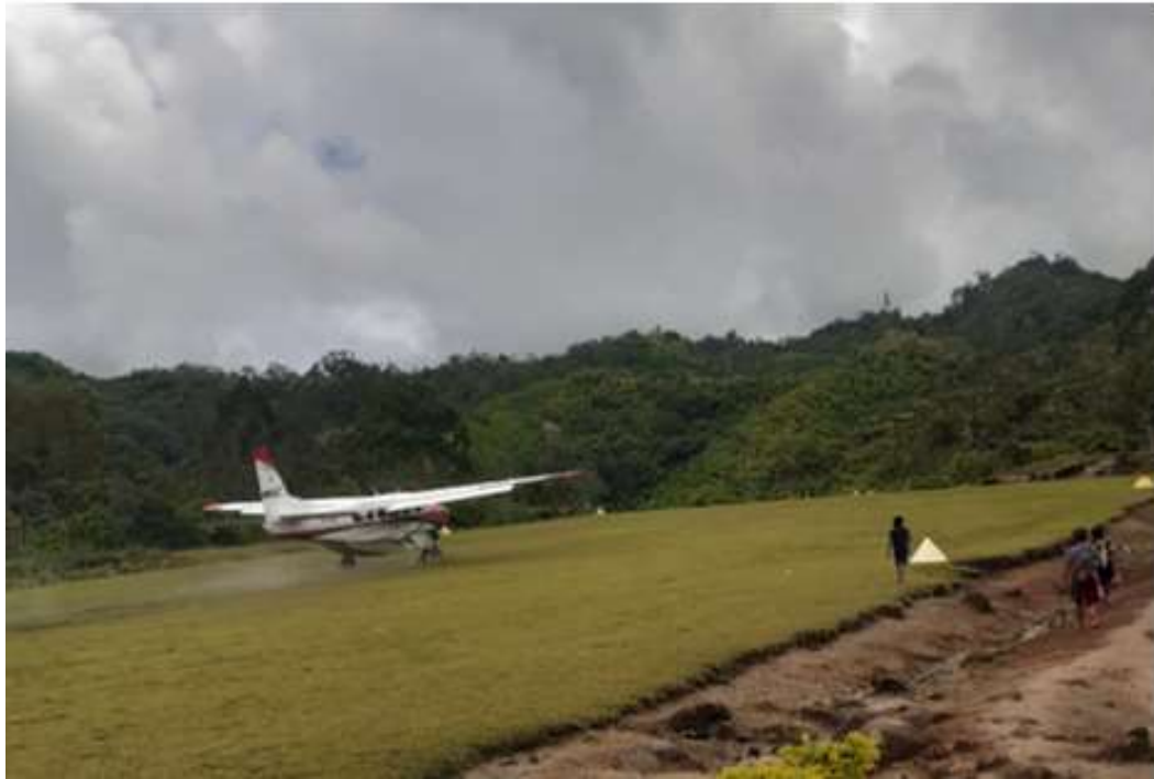
Figure 3: Standing water on airstrip coming out from under the tyres of P2-MAF during landing roll. (Source: Witness)
