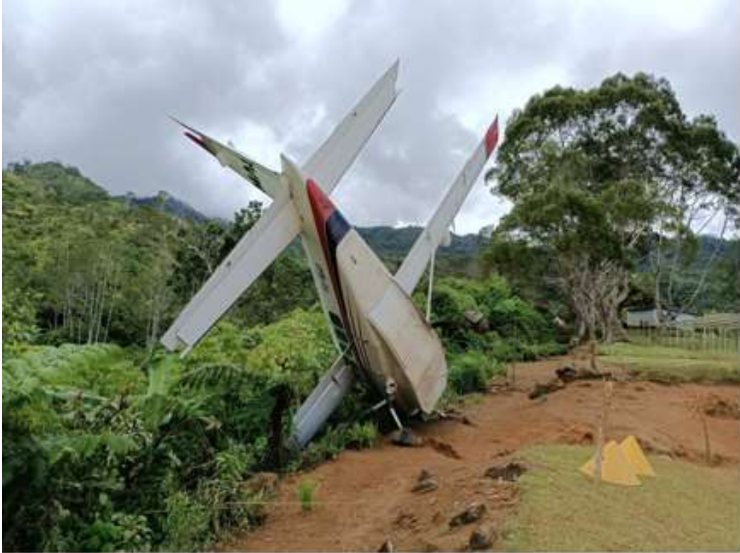
Figure 4: Back view of aircraft tilting on left side into gully at the end of runway.
