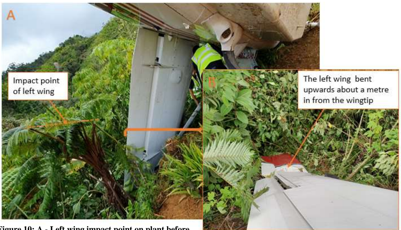
Figure 10: A - Left wing impact point on plant before tilting into gully at the end of runway, B – wing bent upwards about a metre in from the wing tip.
