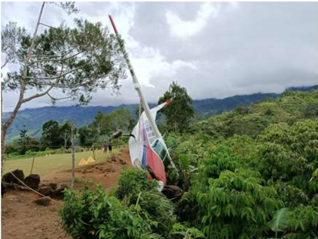
Figure 5: Front view of aircraft tilting on left side into gully at the end of runway.
