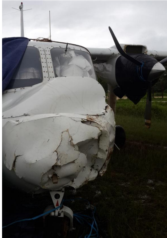
Figure 6: Damage to front of aircraft and the nose landing gear assembly
