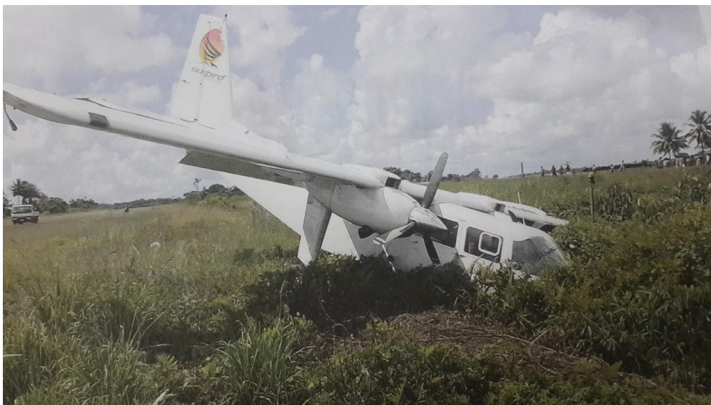
Figure 5: Impact with a side embankment to the left of runway 30
