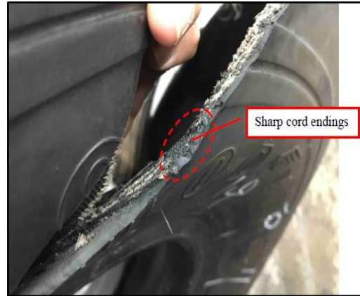
Figure 12: Fractured tyre showing sharp cord endings Source: Tyre manufacturer's report
