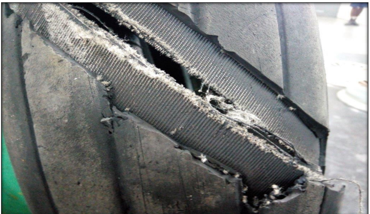
Figure 6: Damage number-two left main wheel tyre
