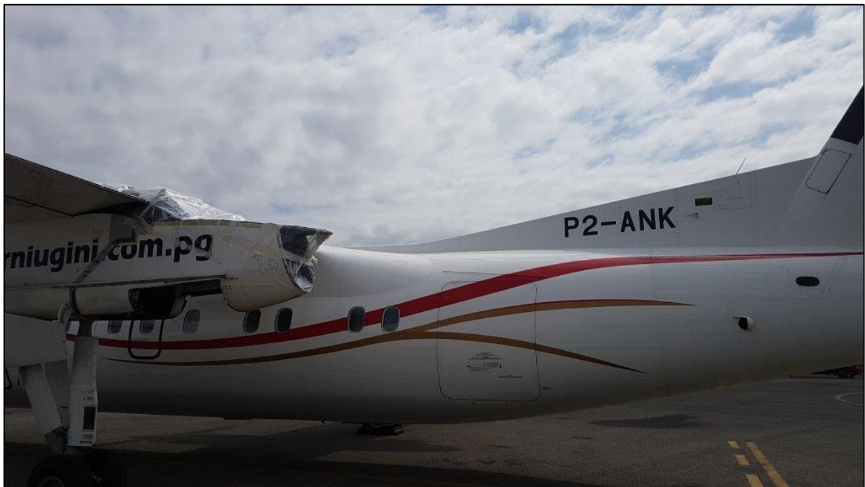
Figure 4. Damaged left nacelle (Wrapped in plastic for protection)
