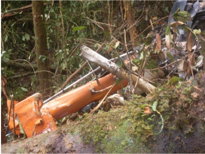
Figure 4: Damaged tail boom
