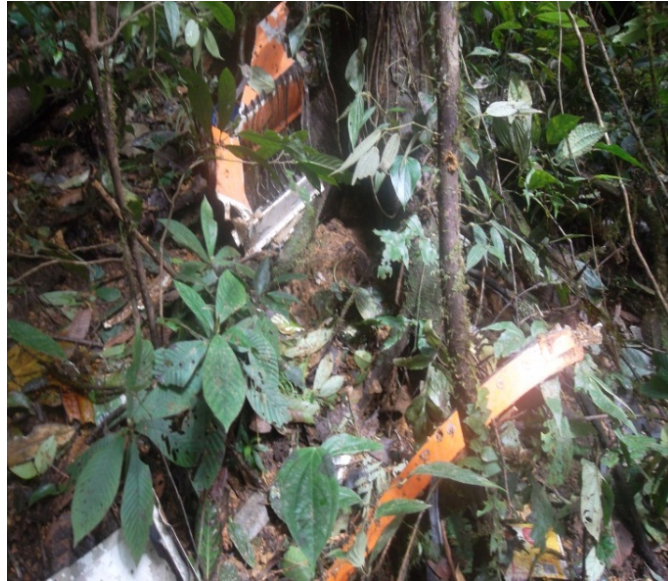
Figure 7: Shows destruction to panels and cowls
