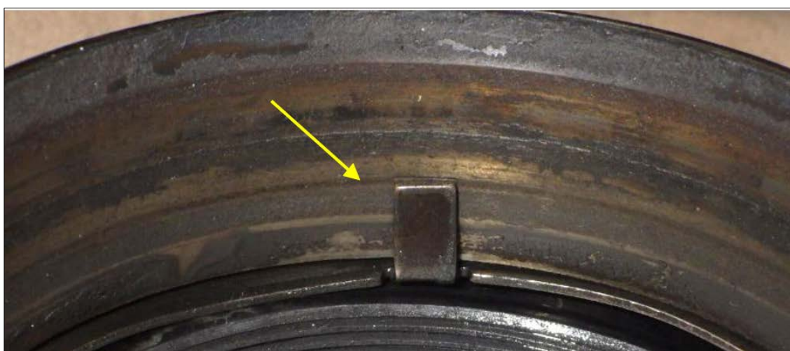
Figure 18: No. 3 bearing rear spacer wear induced by the tang of the key washer
