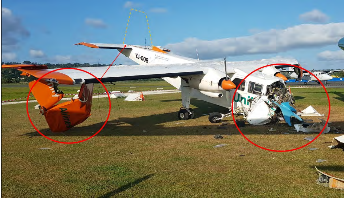
Figure 5: BN-2 Islander, YJ-009 destroyed by the starboard-side of AV71
