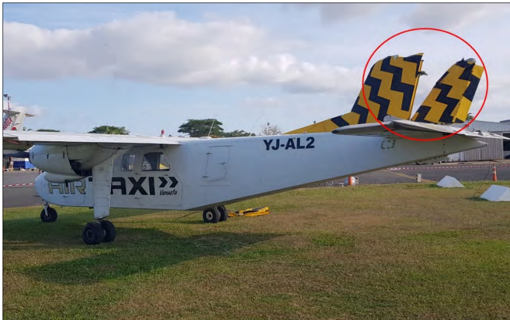
Figure 6: BN-2 Islander damaged by the left side of AV71
