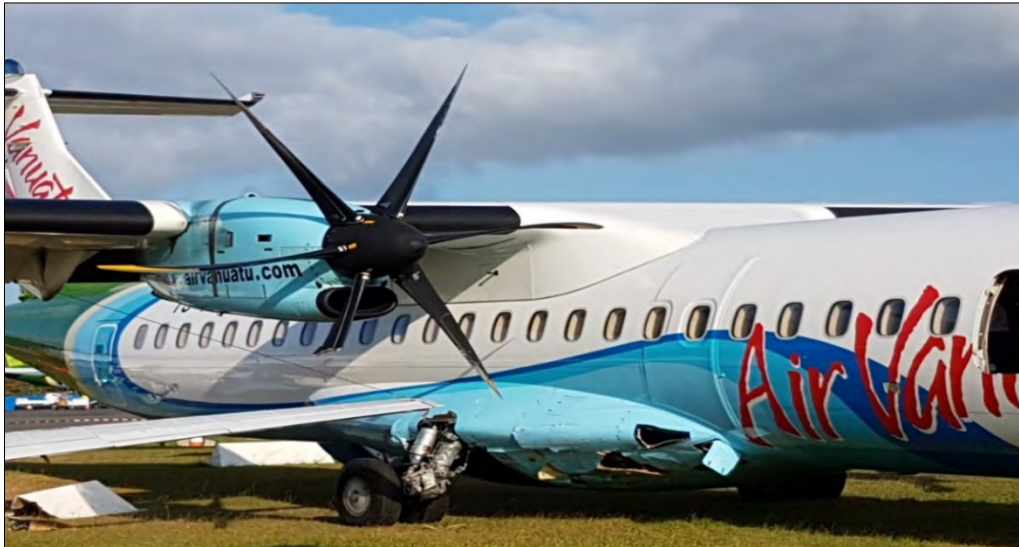
Figure 3: AV71 Right fuselage impact damage
