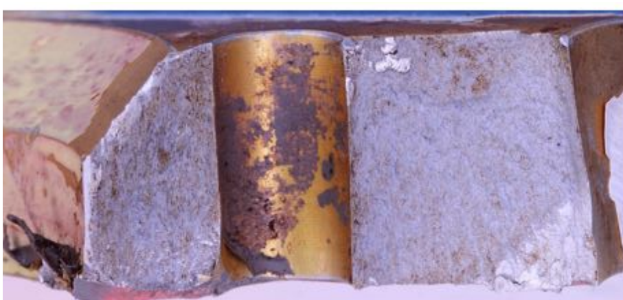
Figure 10: Microscopic view of fracture surfaces (Source ATSB)
