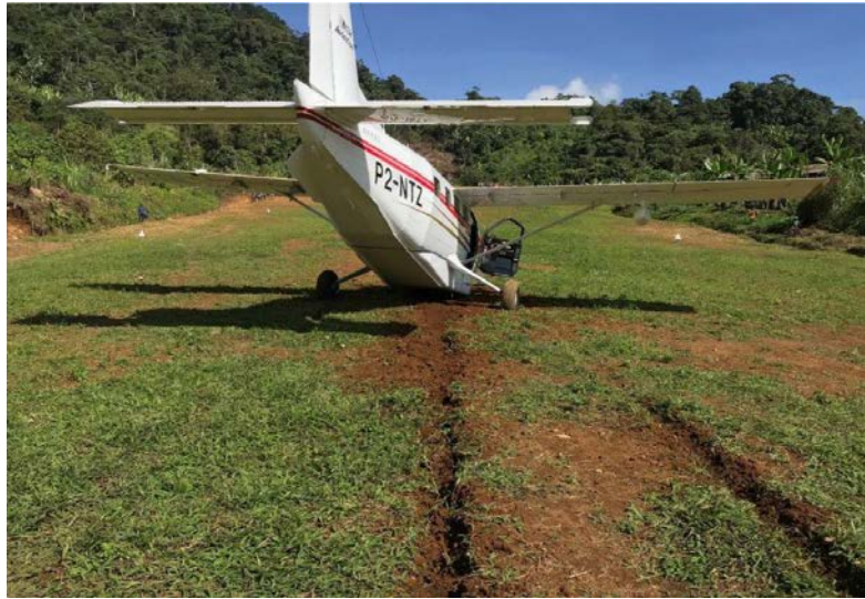
Figure 2: P2-NTZ at Mibu Airstrip showing wheel tracks in strip soft surface
