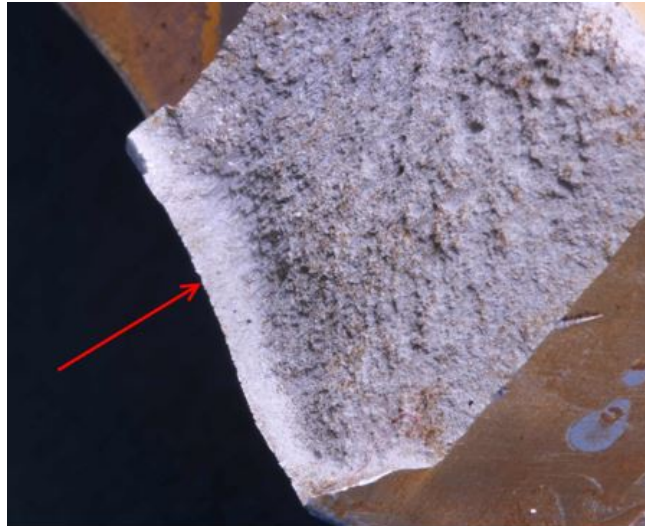
Figure 9: Microscopic view of fracture surface arrow points to shear lip (Source ATSB)
