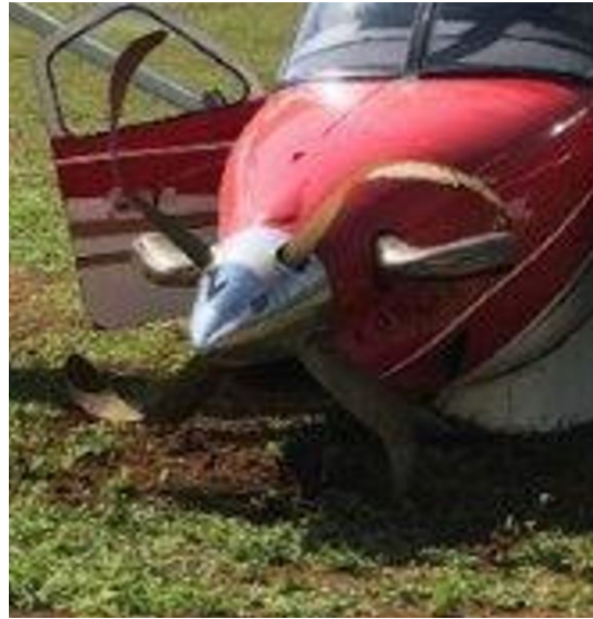
Figure 4: Nose wheel and fork assembly in bog hole Figure 5: Propeller assembly
