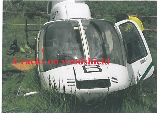
Fig 4: Substantial crack on right windshield
