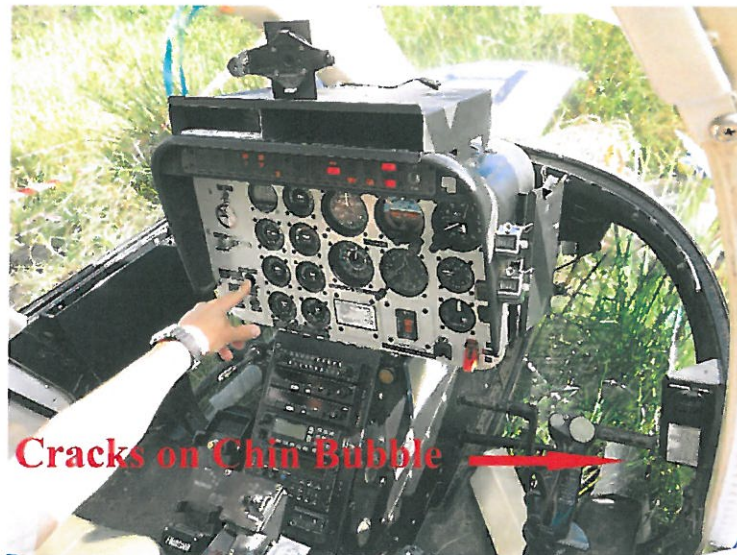
Fig 5: Cracks on chin bubble - right side
