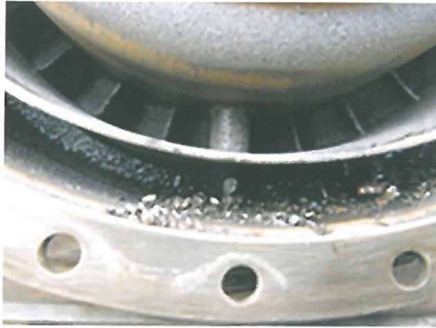
Figure 4: Metallic shavings of the disintegrated turbine
