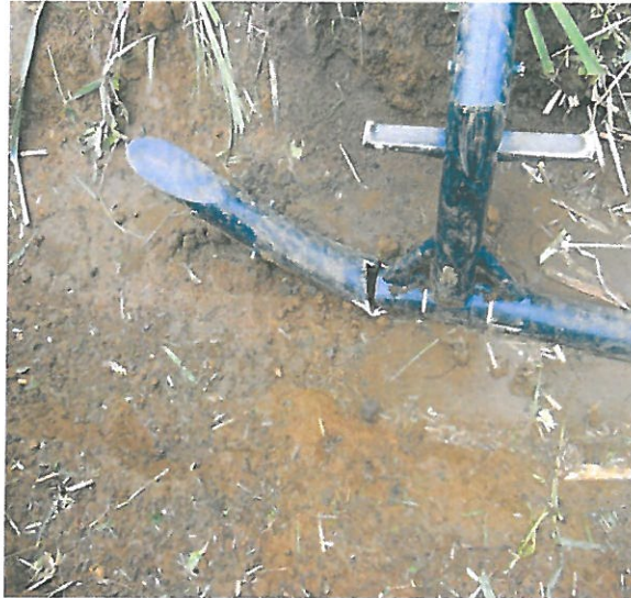
Figure 3: Left landing gear skid damaged as a result of the hard landing
